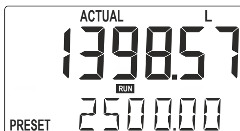
Fig. 6: Example display information during batching process
