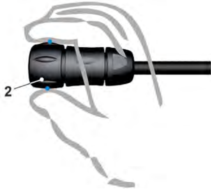
Fig. 25-2 Turning the front ring of the plugs (10polig/18polig)
