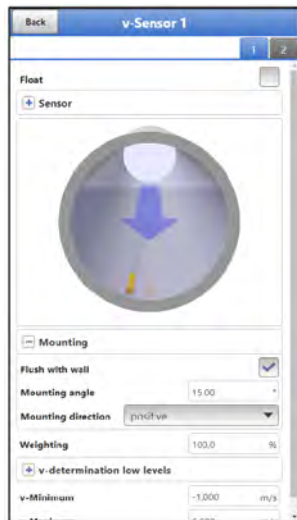
Fig. 40-16 Setting Parameters by Angle Input
