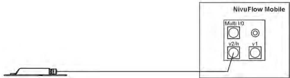
Fig. 26-3 Connection 2nd flow velocity sensor CSM or CSP (if used, DSM-L0 level sensor not connectable)
