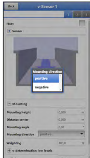
Fig. 40-20 Option to change the Sensor Mounting Direction
