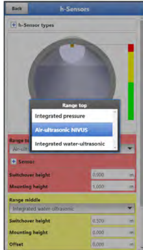
Fig. 40-12 Assignment Level Sensor to Parameterisation Range
