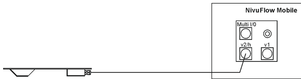
Fig. 26-4 Connection of DSM-L0 level sensor
