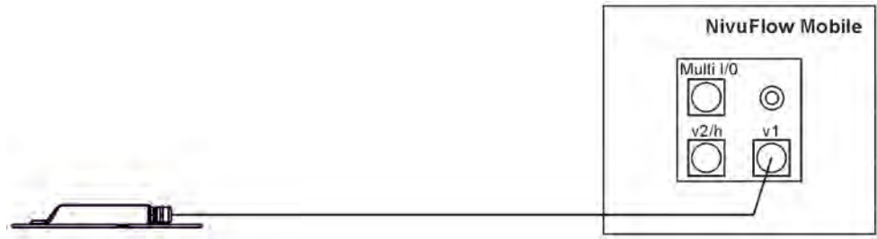
Fig. 26-1 Connection of CSM or CSP flow velocity sensors
