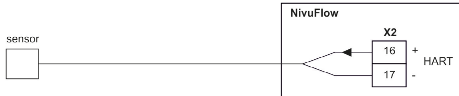
Fig. 16-5 Connection of 2-wire sensor for level measurement
